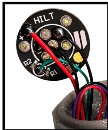
Place the NPXL in the chassis with the lens. The lens should sit flush on the top chassis. Run the wires down through the chassis and out of the chassis under the negative terminal holder. You should now have a mess of wires coming out of your soundboard holder. Please select the wiring diagram for your selected soundboard to continue.
