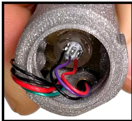
For the ECO NPXL It is recommended to use a 22awg wire for the positive and 28AWG for the negative wires and data line.
