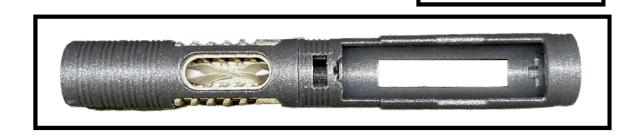
It is very important to check the inside of the saber to make sure no unwanted burs or screw threads are protruding on the inside of the hilt. Some of the screws protruding inside are helpful like the covertech wheel screw. This screw will act as a guide for the chassis orientation to keep the switches and LED's lined up inside the saber while in use.
