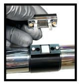
The top of the activation box is held on with a magnet. Pull the top of the activation box off to reveal the screws holding the activation box. Check inside the saber to see if they are sticking out. If they are, you may need to remove 2mm of length from the screws. These can potentially destroy the switches on the PCB if they are too long.
